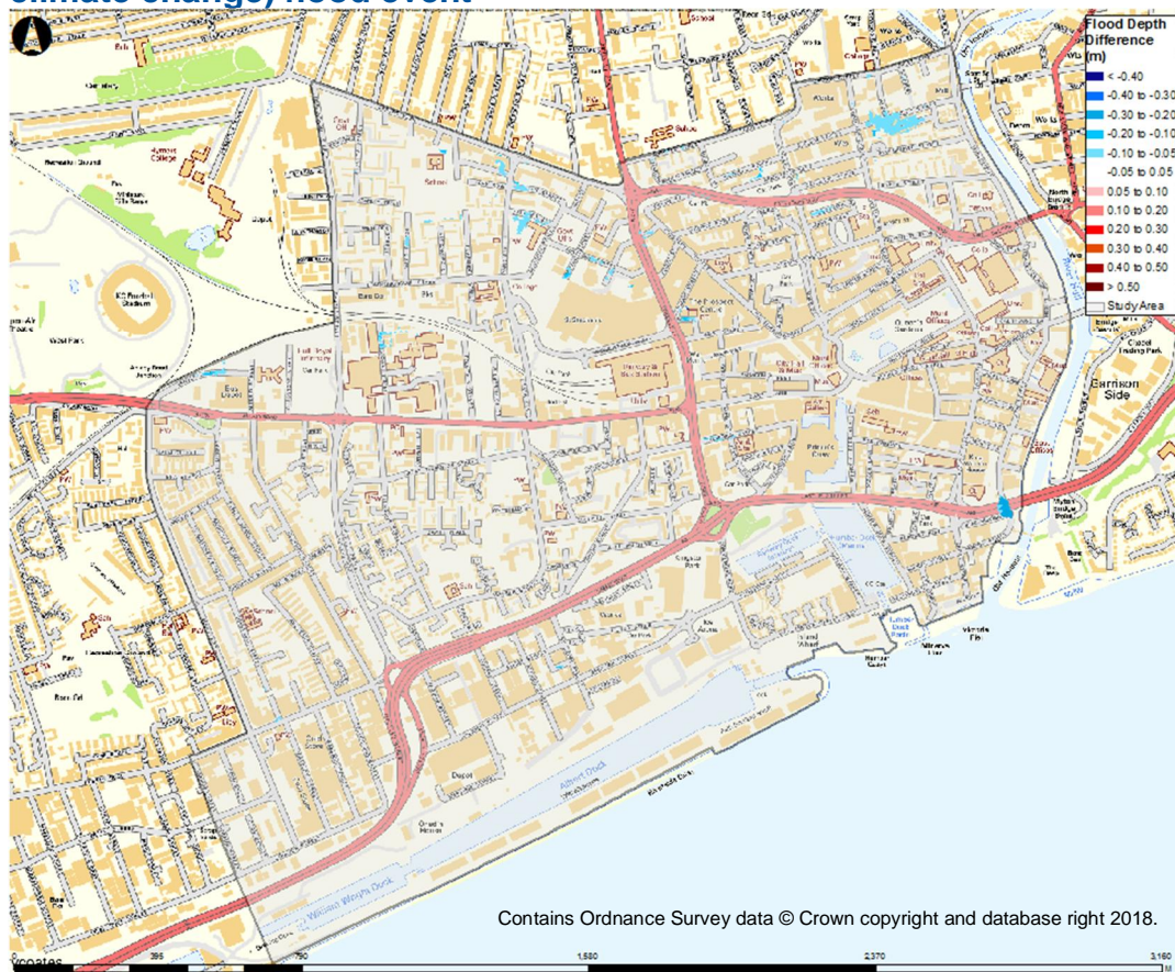
Figure 3-8: FEH13 sensitivity (flood depth differing for a 1 in 100-year plus climate change) flood event
